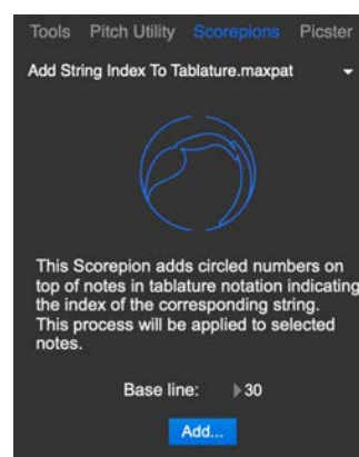
Figure 15. GUI of the Add String Index To Tablature Scorepion for the MaxScore Editor.
