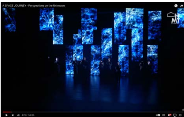
Figure 9. A frame from the live stream of the premiere showing the performance of Solaris I. The eight singers holding their iPads are positioned in front of the LED video wall panels mounted on a computer-controlled fly system.
