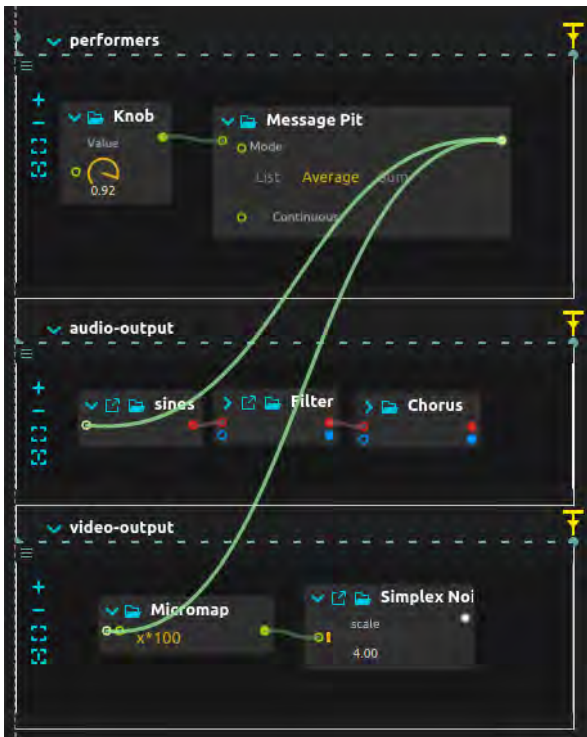
Figure 5: A single client’s input data will be broadcast to all the machines in the audio and video groups.
